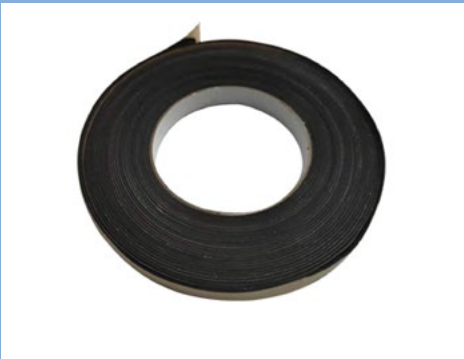
RUBBER STRIP Provides sound reduction and friction reduction between the joist and the decking material.
