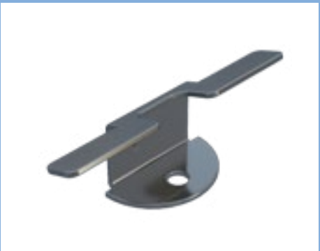
ALUMINUM JOIST STARTER CLIP 3/8" TO 7/16" High clip for bottom thickness of decking slot 9-11mm.
